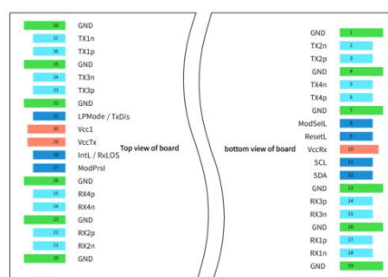
Figure4:QSFP112 Module contact assignment
